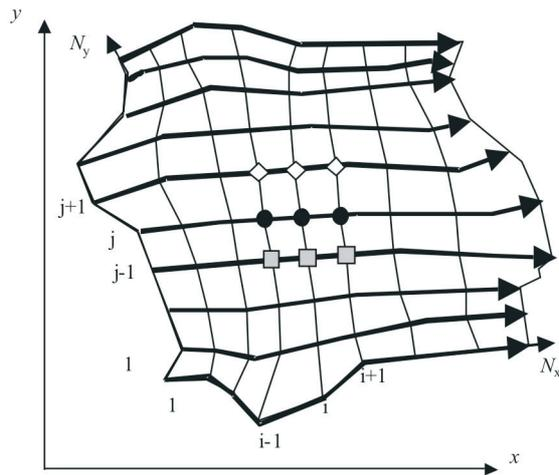
Figure 2. Grid for a basin of irregular boundary. The symbols (□), (◇) and (○) indicate the position of variables are known, variables are solved and variables extrapolated respectively.
